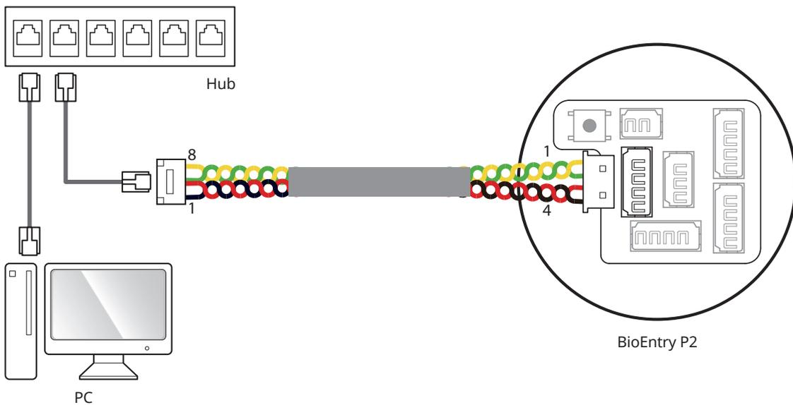
**LAN connection (connecting to a PC directly)**
