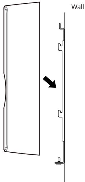
**3** Connect BioEntry P2 to the bracket by rotating the product fixing screw.
